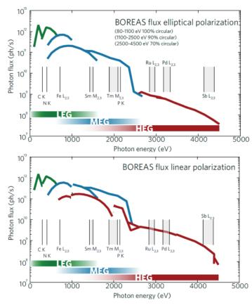
**Figure 1.** Photon flux measured on a silicon diode after the last optical element of the BOREAS beamline.
