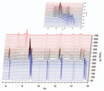
**Figure 2**. Reduction of  $LaCoO_3$  to  $La_2O_3$  + Co under 5 %  $H_2$ /He gas flow. The transition is passing through a brownmillerite intermediate. Each temperature scan was collected in 8 minutes.
