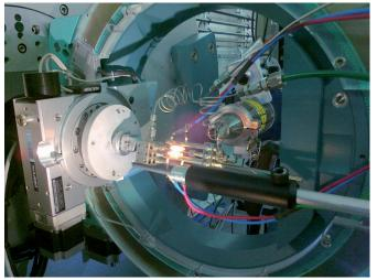
**Figure 3.** In situ reaction capillar flow cell mounted on the PD diffractometer. The shiny color is due to the radiation of the heating elements.
