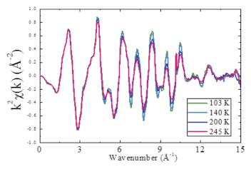
**Figure 1.** EXAFS signal, weighted in  $k^2$ , of  $YFe_2O_4$  at different temperatures. Spectra were taken in 10 min using the continuous scan mode.
