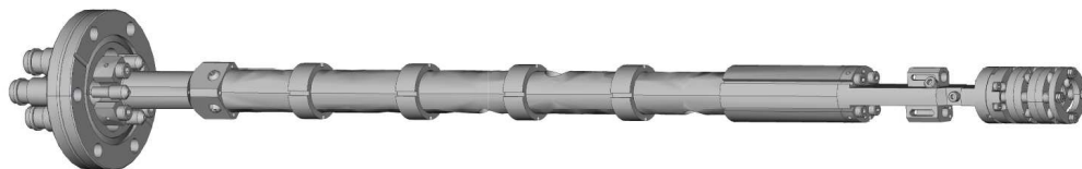
Figure 10. Fluorescence diode assembly designed and built at ALBA.
