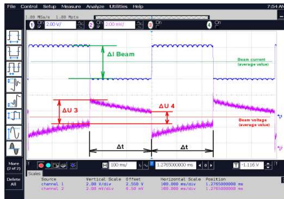
RF power (blue) and collector voltage (pink)
