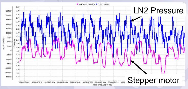
1 bar LN2 supply pressure variation leads to significant tuner motion
