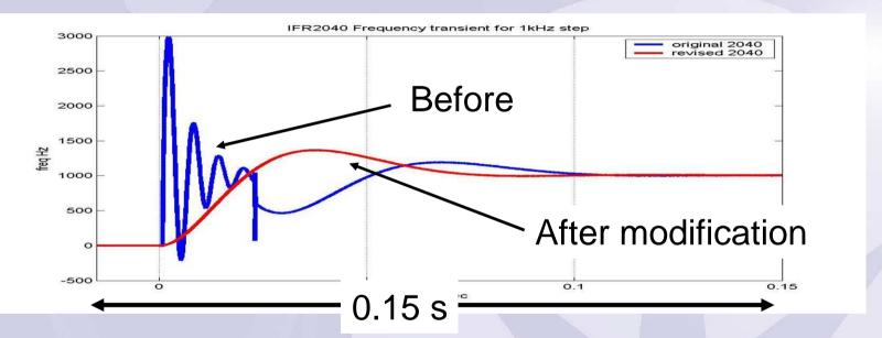
Frequency transient before and after MO firmware upgrade
