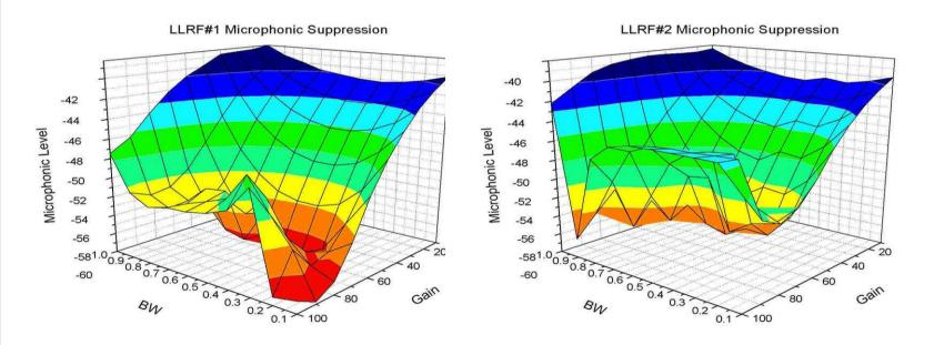
Measured suppression of 2 kHz microphonics (applied via cavity simulator)
