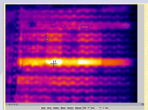
Thermal distribution of water load indicates blocked channel
