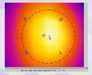
Thermal distribution with cavity detuned (73 kW, no beam)
