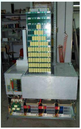
>The HV power supply of each IOT is a switched mode power supply.
