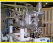
Vacuum tests on the cryomodule at ELETTRA, just before installation
