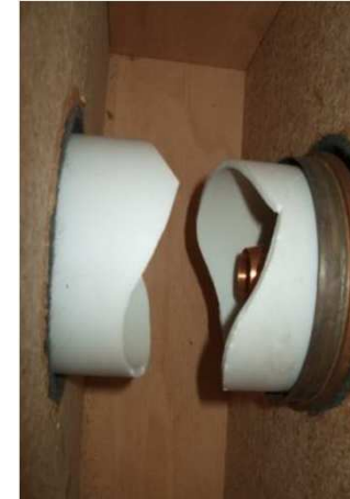
Broken ceramic window of a klystron
