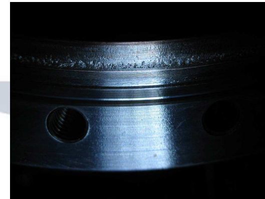
Figure 2: Cavity flange for window damper. Bad quality: bumpy
