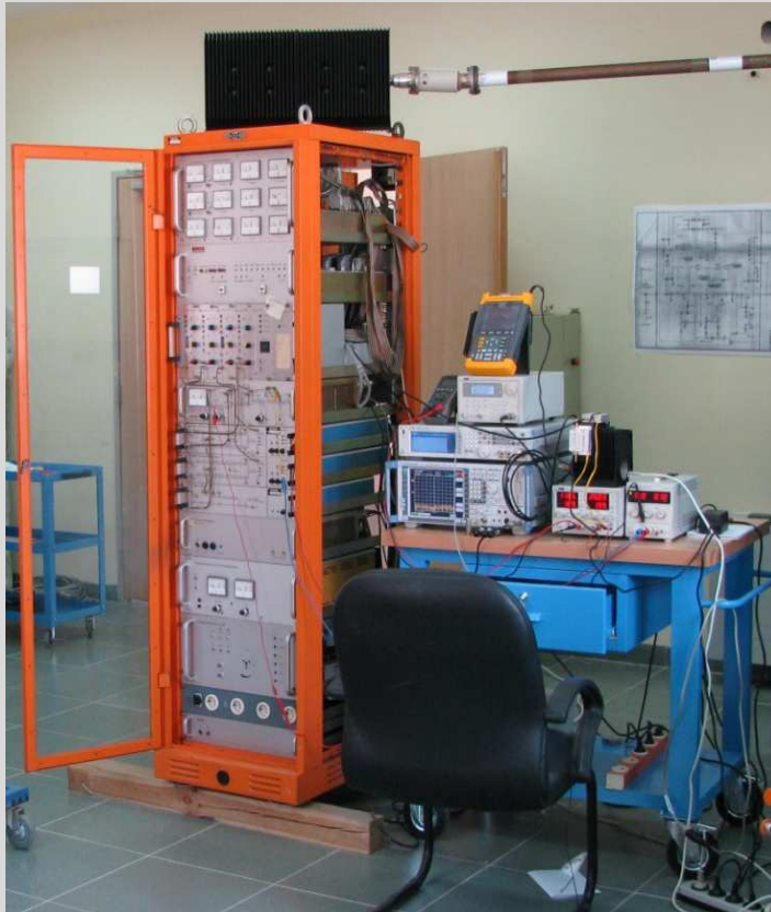
Booster LLRF (from BESSY I) tested in the RF lab
