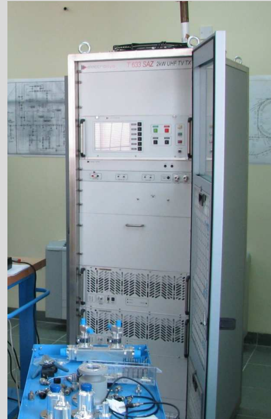
The new 2kW Solid-State amplifier as replacement for the old klystron used in BESSY I
