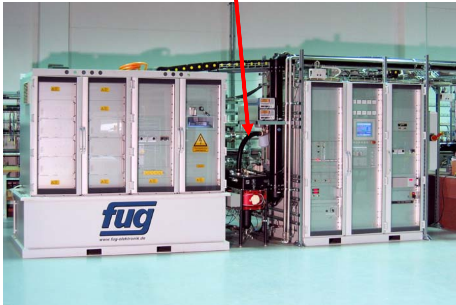
500 MHz 80 kW transmitter at the MLS
