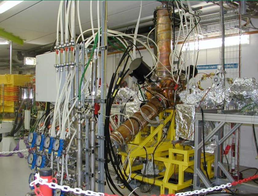
EU cavity at the MLS storage ring 360° view of the MLS storage ring
