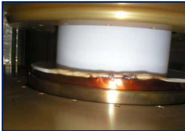
LEP kovar based coupler overheated
