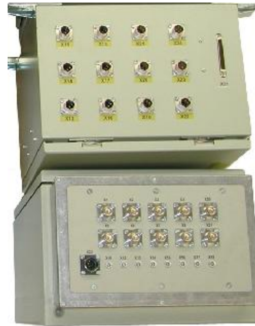
Down Converter Box
