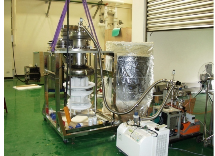
LN2 Cold Shock for vacuum leak check
