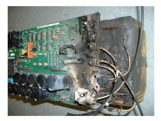
Cause = loose electrical connection (after 16 months operation !) ESLS 04 Daresbury Laboratory
