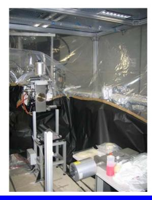
This required to break the cavity vacuum. A clean area was therefore created inside the storage ring tunnel. The replacement followed clean room procedures and was done by CEA and Elettra staff. The field performance of the cavity has not been affected by this intervention.
