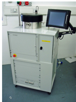
Reflow Vacuum Hotplate With Formic Acid Clean. Wafer sizes up to 200mm. On site, awaiting installation.
