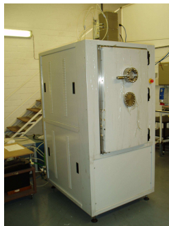
Indium Evaporator. Wafer Size up to 200mm.
