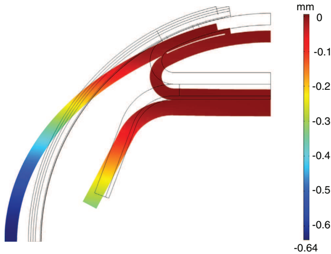
FIG. 17. Maximum displacement of the beam screen in the horizontal direction during a magnet quench.
