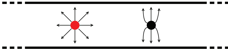
FIGURE 3.1. The Electric field lines of a charge (red) get squeezed in the direction of motion when approaching the ultrarelativistic limit (black).
