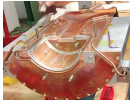
Figure 3: Liner clamped on the tooling during the soldering process of the cooling tubes.
