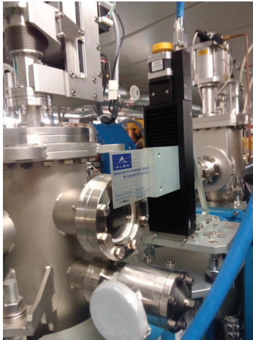
Figure 5.13: Motorized Hartmann Mask mounted close to the extraction window of FEo1.
