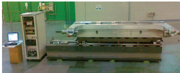
Figure 4: Picture of the new Hall probe bench developed at CELLS. This bench is specifically conceived to measure closed big magnetic structures.
