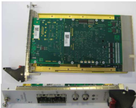
Figure 15: New PMC-FPGA board from IOxOS (side and front views)
