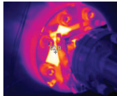
Figure 2: Infrared image of the beam pipe flange.
