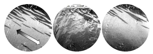
Magnetic microscopy images (Field of view 50um, XMCD-PEEM at Mn-L3) of the LSMO thin film at the same location: from the left with +240 V, -240 V and again +240 V voltage applied across the piezoelectric substrate. The arrow indicates the direction of the greyscale magnetic contrast.
